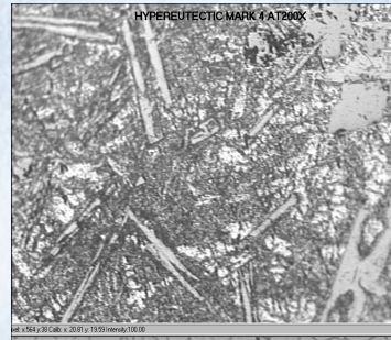
Al-20Si-0.5Mg-1.2Fe-0.03 Be stir cast
