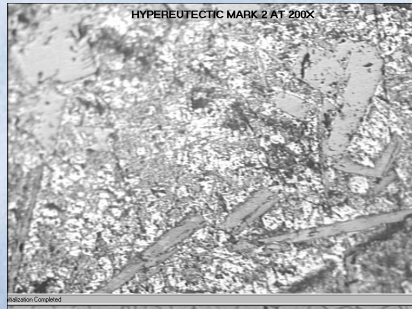
Al-20Si-0.5Mg-1.2Fe stir cast
