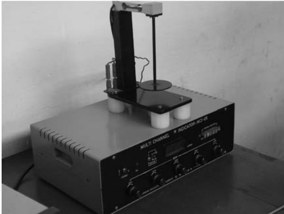
Fig. C.51 Typical set-up for strain measurement
