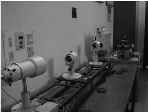
Fig. C.23 Autocollimator for the measurement of straightness
