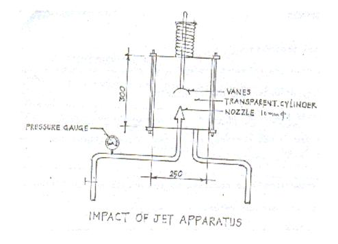
**Experimental set up**: The experimental set up primarily consists of a nozzle through which a water jet imerges vertically in such a way that it may be conveniently observed through the transparent cylinder. It strikes the target vane positioned above it. The force applied on the vane by jet can be measured by applying weight to counteract the reaction of the jet. Vanes are interchangeable i.e. flat, inclined or curved vane.
