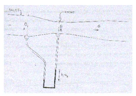
at the throat will become greater than that at the inlet section, according to continuity equation. The increase in the velocity of flow at the throat result in the decrease in the pressure at this section. A pressure difference is created between the inlet section and throat section which can be determined by
