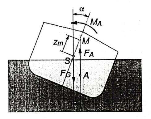
Figure: Metacenter and Metacentric Height. FA=Buoyancy Force, FG=Dead weight. S = Center of gravity, A = center of buoyancy, M = metacenter location, zm = distance between center of gravity and metacenter
