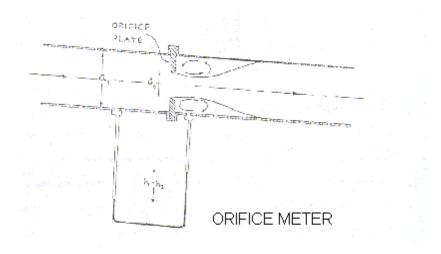
An orifice meter consists of a flat circular plate with a circular hole called orifice which is concentric with the pipe axis. The upstream face of the plate is beveled at an angle lying between 30 and 45. The plate is clamped between the two pipe flanges with beveled surface facing downstream. The pressure taps are
